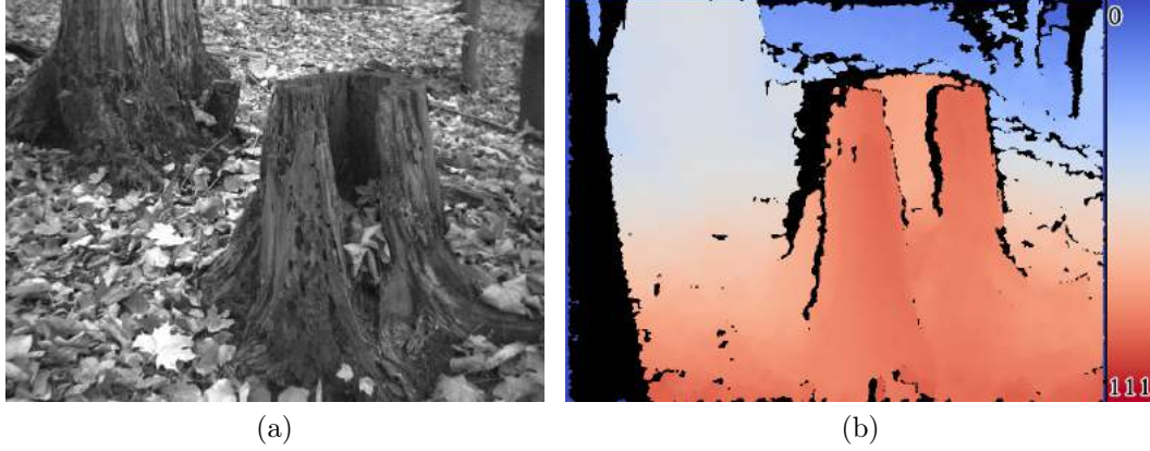
Figure 9: Example for (a) left camera image and corresponding disparity map.
