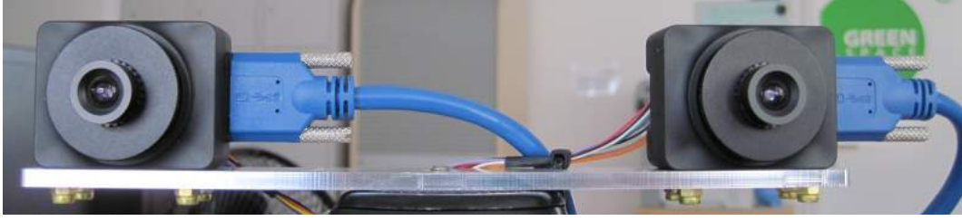
Figure 6: Example for standard epipolar geometry.
