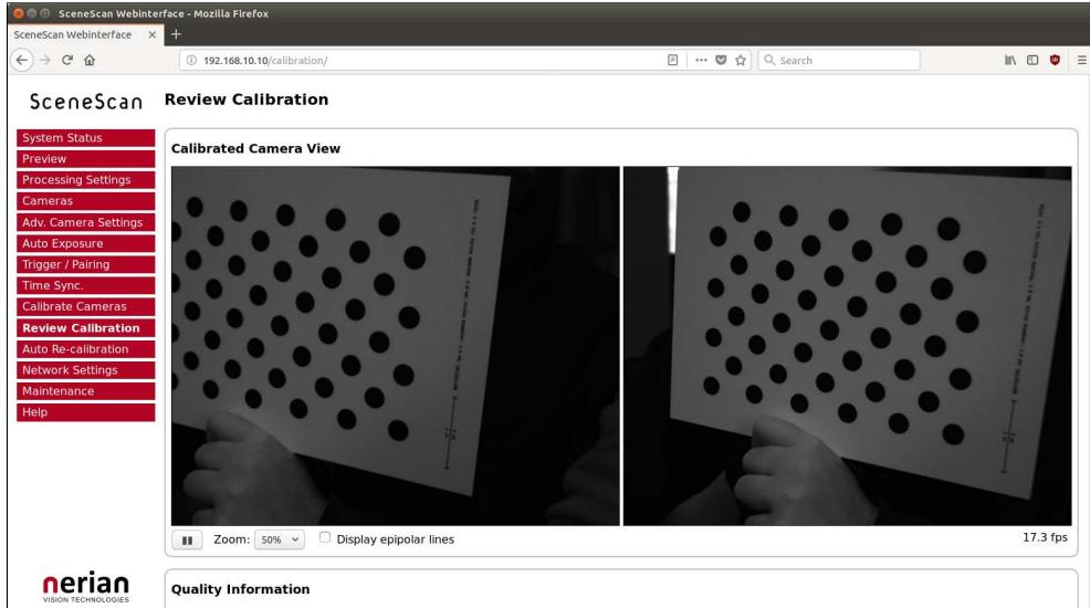
Figure 23: Screenshot of configuration page for reviewing camera calibration.
