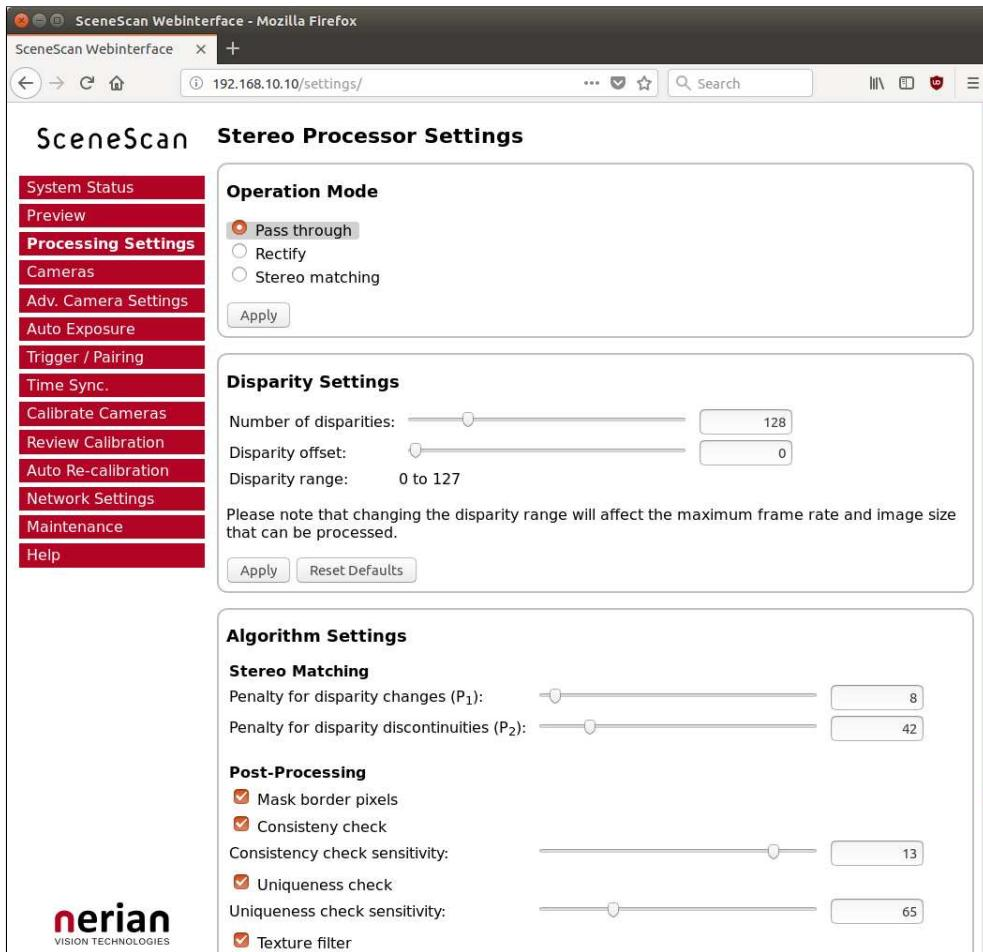
Figure 14: Screenshot of configuration page for processing settings.
