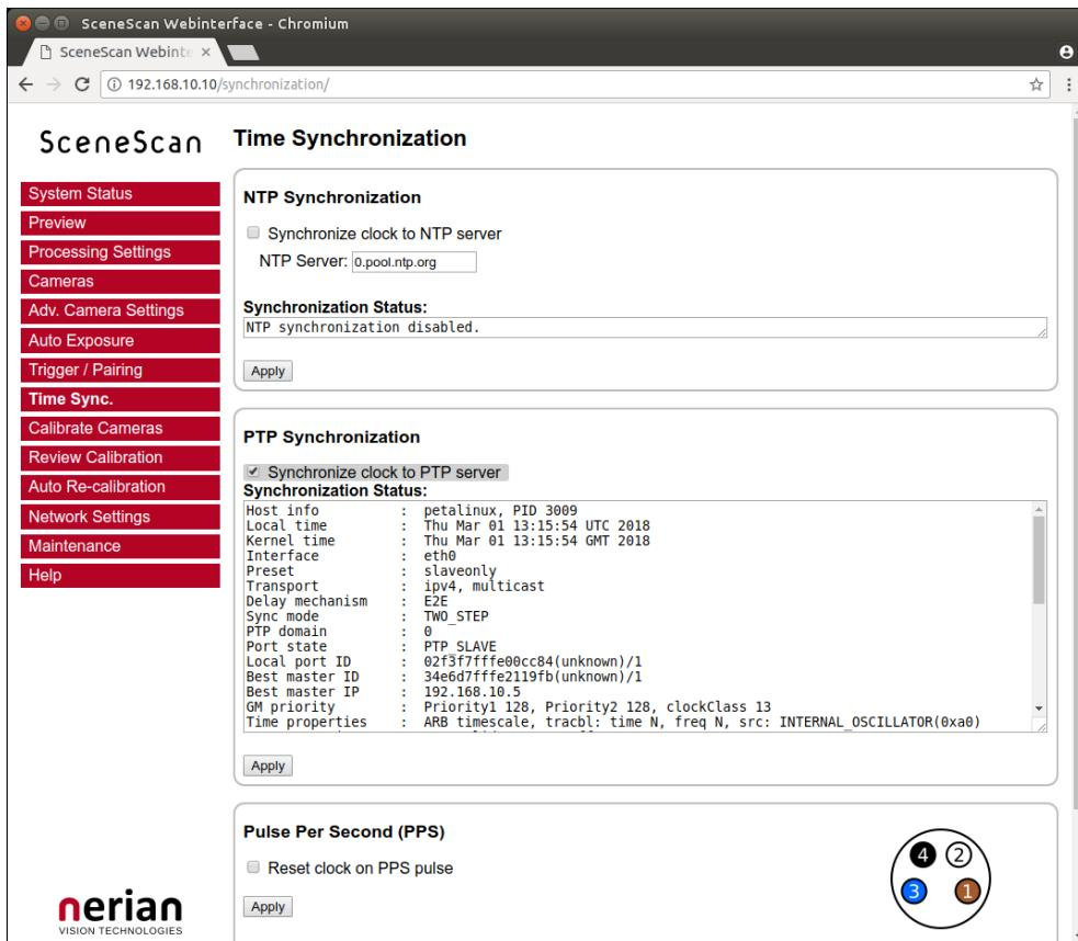
Figure 19: Screenshot of configuration page for time synchronization.
