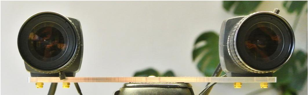
Figure 8: Example for valid stereo camera setup.
