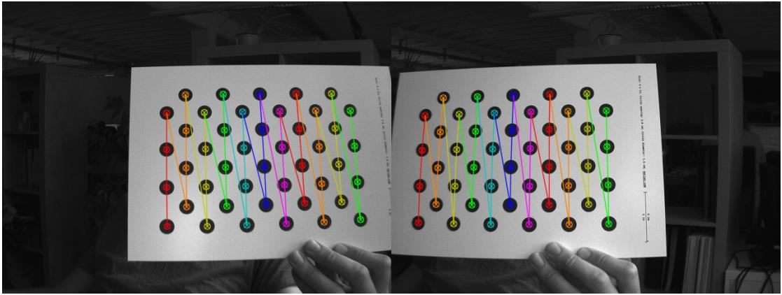
Figure 22: Example calibration frame with detected calibration board.
