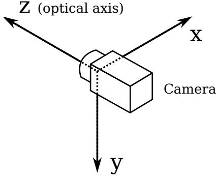
Figure 11: Coordinate system used for 3D reconstruction.
