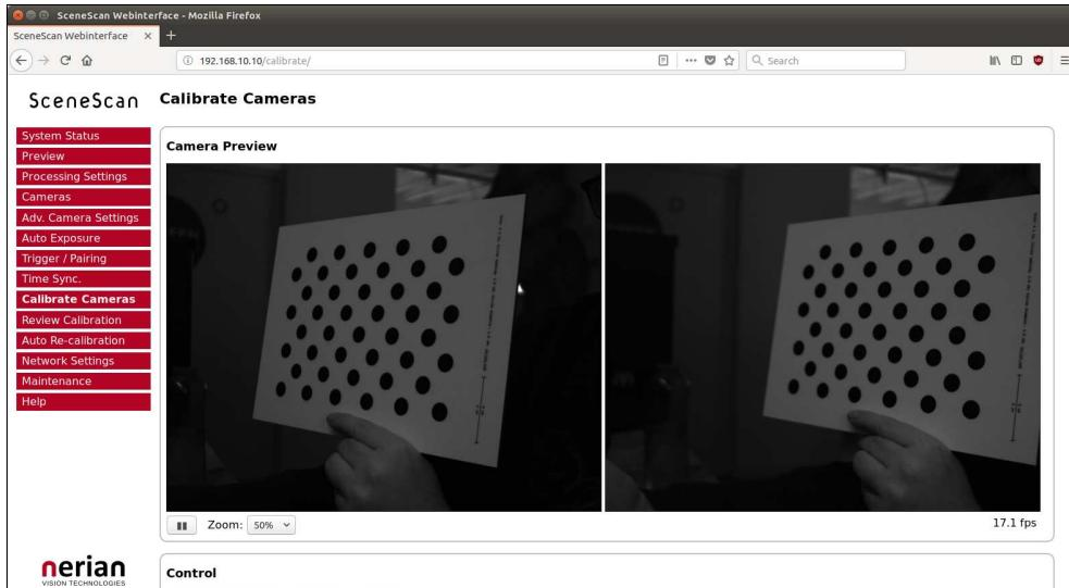
Figure 20: Screenshot of configuration page for camera calibration.
