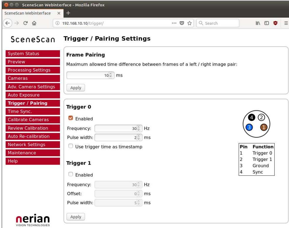
Figure 18: Screenshot of configuration page for trigger settings.
