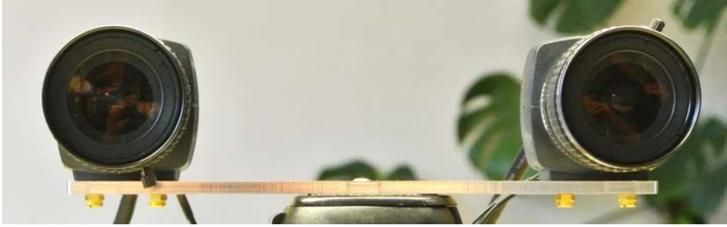
Figure 8: Example for valid stereo camera setup.
