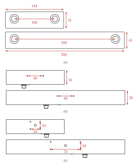
Figure 1: (a) Dimensions and (b-c) placing of mounting holes for 10 cm and 25 cm versions of Karmin2. All measurements are provided in millimeters.
